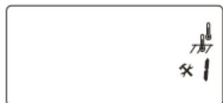
The sensor mode is detected and initialised automatically. If the floor sensor cable is connected, it operates in floor sensor mode <
